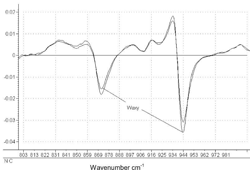
Fig. 4. First derivative spectra of the samples P8 and P9 in the [800\text{--}1000\text{ cm}^{-1}] spectral region.
